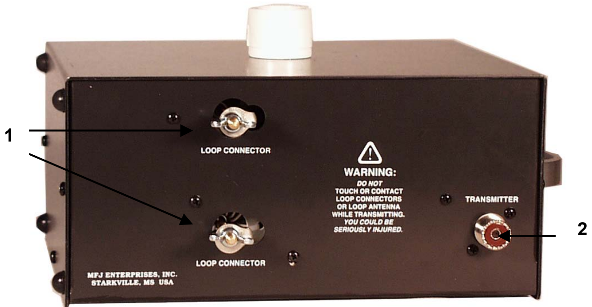
Figure 5 MFJ-936B Loop Tuner ™ Rear Panel Connections
