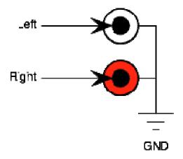
For each of the three ports, Port 1, Port 2, and Common, the 1/8" stereo jack pinout is as follows:
