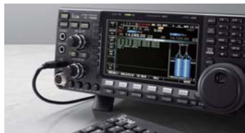
Installation example of USB keyboard
