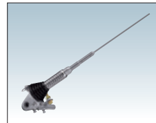
AH-2b ANTENNA ELEMENT A 2.5m long antenna element for mobile operation with the AH-4. All bands between 7–54 MHz can be matched.
