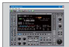
RS-BA1 IP REMOTE CONTROL SOFTWARE For IP remote transceiver control from a PC.
