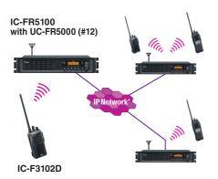
When using the IC-F3102D series in dPMR Mode 2 multi-site system, the IC-F3102D can communicate with other dPMR radio users working with other repeater sites on the network.
