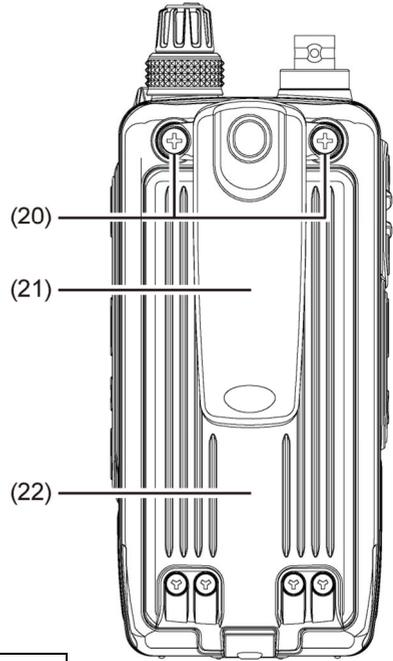
**All rubber covers must be closed and the battery pack installed for the receiver to be waterproof (IPX5).**
