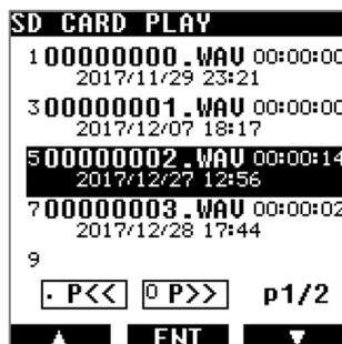
2. Select the desired recording and press [ENT] to start the playback. [PLAY] will blink at the top of the screen during playback.
