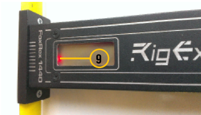
9. Battery charge indicator.
