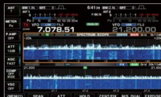
Dual scope example (Vertically aligned)
