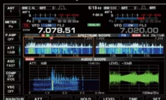
Mini dual spectrum scope and audio scope
