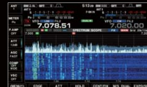
Spectrum scope with waterfall (wide screen setting)
