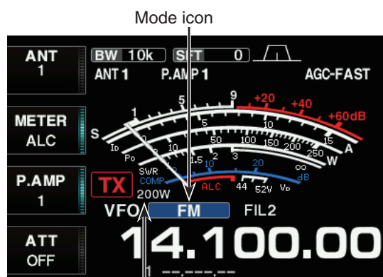
TX power readout
