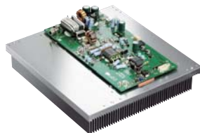
PA unit and large heat sink
