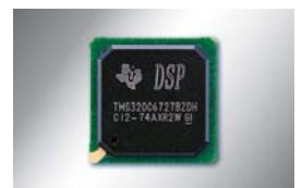
Tx/Rx DSP: TMS320C6727 Internal Clock: 250MHz 32-bit floating point Floating point calculation: 1800MFLOPS
