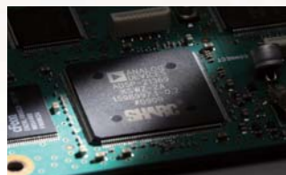
<DSP unit> ADSP-21369 Internal clock speed: 333MHz 32-bit floating point DSP Max. performance: 2000MFLOPS
