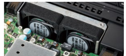
Thermostatically-controlled Dual Internal fans
