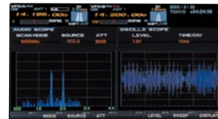
■ Audio Scope/Oscilloscope Display
