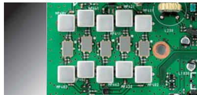
Five roofing filters
